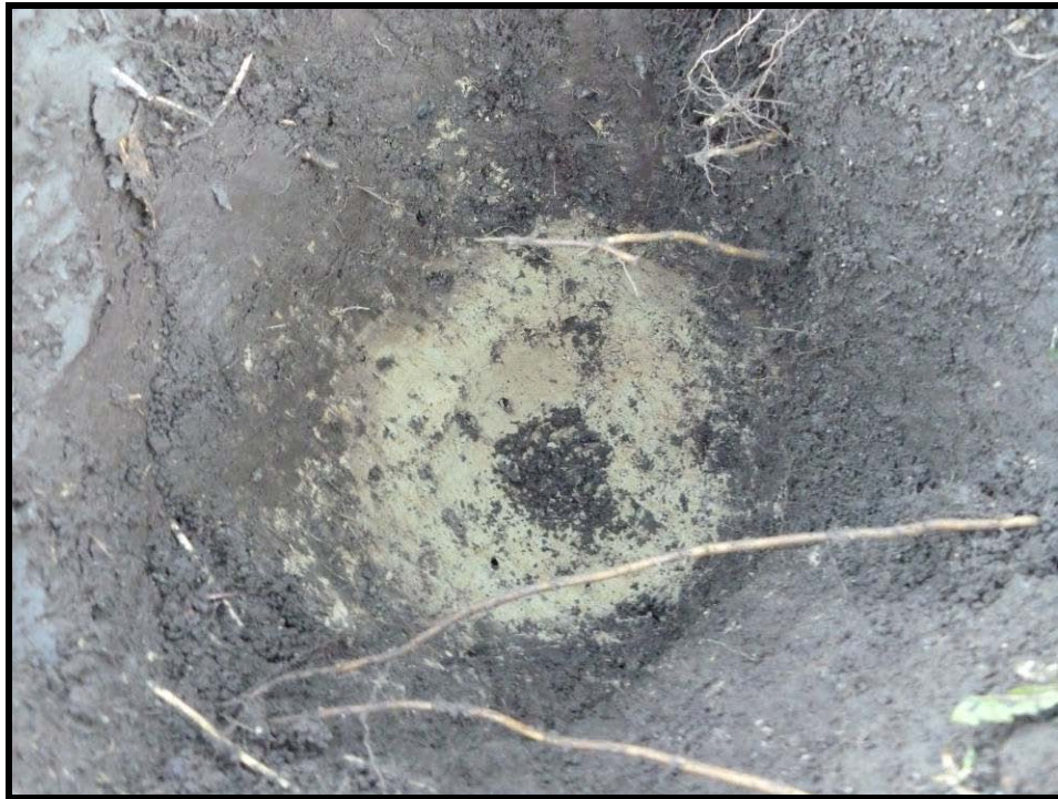
Plate 8: Typical Test Pit, Excavated to Subsoil
