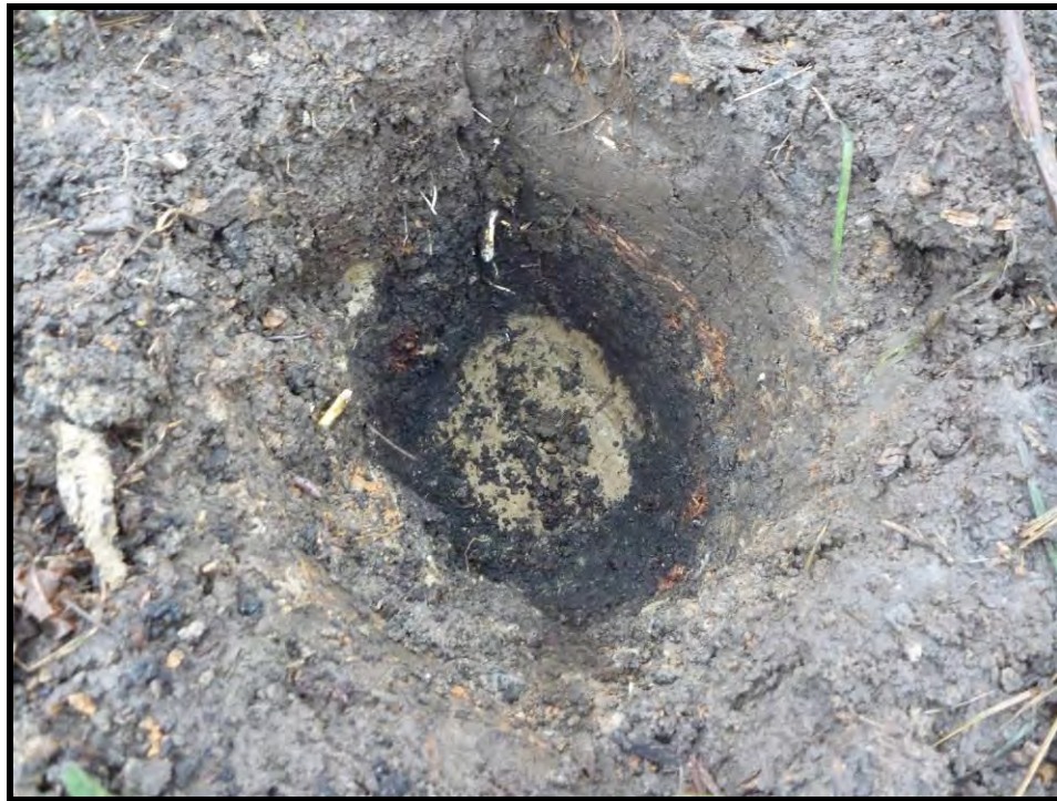
Plate 5: Typical Test Pit, Excavated to Subsoil
